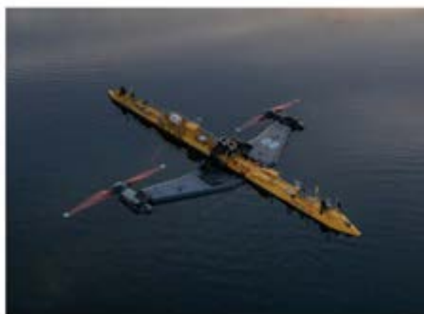
Figure 2. Ocean energy devices: CorPower Ocean’s point-absorber WEC (left) and Orbital Marine Power’s floating tidal device (right).
